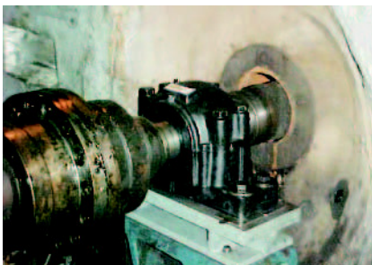
Bearing arrangements in fans and ventilators
