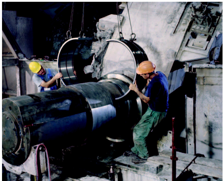
Fitting of a large split spherical roller bearing
