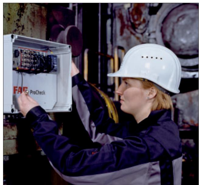
Gearbox monitoring on a hot rolling line
