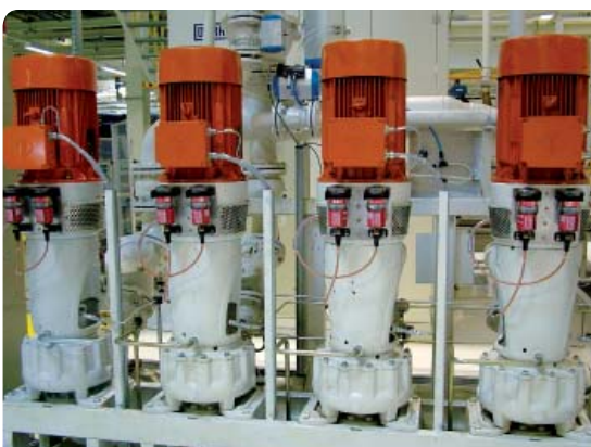
Lubrication system: 2 STAR CONTROL 120 cm 3 each
